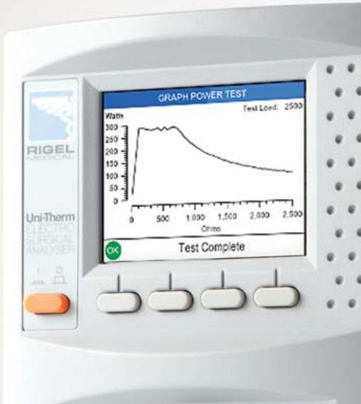
Using its unique and industry leading load bank to simulate human tissue behaviour, the Rigel **Uni-Therm's** bespoke current measurements technology makes it an extremely versatile test instrument for calibrating and performance testing of all high power electro-surgical instruments on the market.
